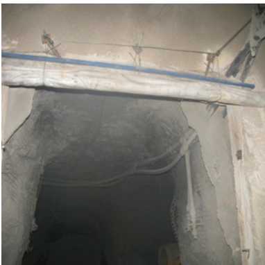
FIG 4 - Original design of a QBC access curtain with chain hangers (MIM, 2013)
